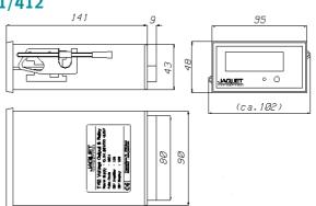
Rail DIN 4622713 (EN 50022) or mounting plate to DIN 43660 (46121)
